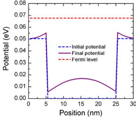
Fig. 2. Potential profile and Fermi level of the 20 nm/10 nm InGaAs/InGaAlAs (10% Al) superlattice uniformly doped by  $5 \times 10^{17} \text{ cm}^{-3}$ . Both the initial potential and the final potential after band bending due to charge transfer are shown (color figure online).
