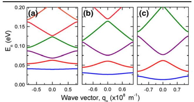
Fig. 1. Dispersion curves of minibands in InGaAs/InGaAlAs (10% Al) superlattices with well/barrier widths of (a) 20 nm/20 nm, (b) 20 nm/10 nm, and (c) 20 nm/5 nm (color figure online).
