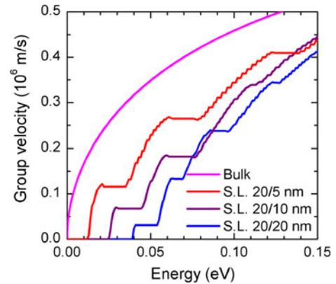
Fig. 4. Electron group velocity in the cross-plane direction of InGaAs/InGaAlAs (10% Al) superlattices with three different barrier widths in comparison with that of bulk InGaAs (color figure online).
