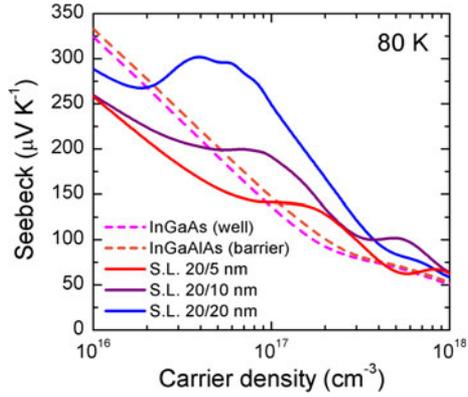
Fig. 5. Seebeck coefficient in the cross-plane direction of InGaAs/InGaAlAs (10% Al) superlattices with three different barrier widths in comparison with that of bulk InGaAs and InGaAlAs (10% Al) as a function of carrier density at 80 K (color figure online).
