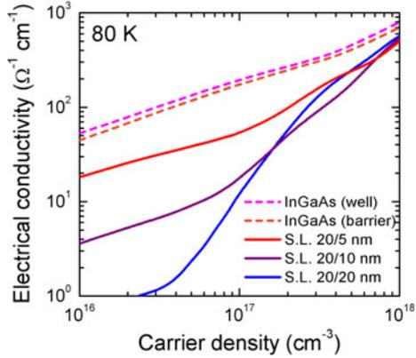
Fig. 6. Electrical conductivity in the cross-plane direction of InGaAs/InGaAlAs (10% Al) superlattices with three different barrier widths in comparison with that of bulk InGaAs and InGaAlAs (10% Al) as a function of carrier density at 80 K (color figure online).
