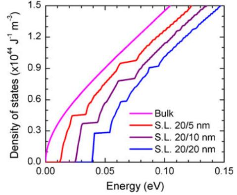
Fig. 3. Density of states of InGaAs/InGaAlAs (10% Al) superlattices with three different barrier widths in comparison with that of bulk InGaAs (color figure online).
