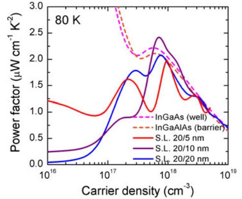
Fig. 7. Power factor in the cross-plane direction of InGaAs/InGaAlAs (10% Al) superlattices with three different barrier widths in comparison with that of bulk InGaAs and InGaAlAs (10% Al) as a function of carrier density at 80 K (color figure online).
