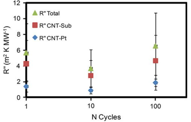
Fig. 7. Effect of thermal cycling from 30°C to 200°C on CNT film boundary resistances.  $N$  is the number of cycles.
