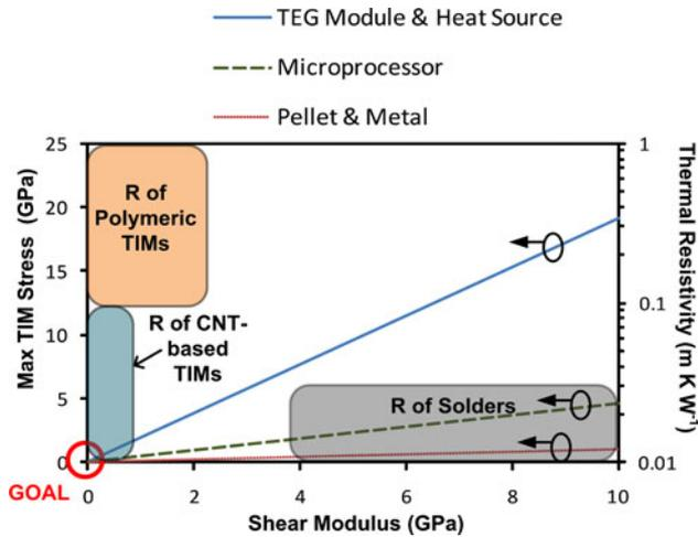
Fig. 1. Lines: maximum TIM stresses ( $\sigma$ ) in TEG and microprocessor applications based on values from Table I. Polymeric TIMs range from particle-filled oils to epoxies, with shear modulus in the 0 GPa to 2 GPa range. The modulus of solders range from roughly 4 GPa (e.g., pure In) to 10 GPa (e.g., hard solders). Boxes: thermal resistivity ( $R$ ) values (right axis, log scale) for CNT-based TIMs, polymeric TIMs, and solders.
