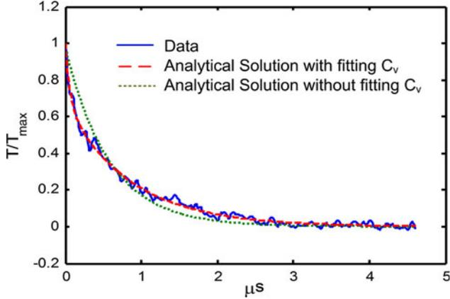
Fig. 6. Thermal response trace data (*solid*) and best-fit analytical solution (*dashed*) for CNTs grown on SiGe film measured with the nanosecond thermoreflectance system.  $T/T_{\max}$  is normalized surface temperature. The *dotted line* shows a poor fit when the CNT layer is fitted as a lumped total resistance.
