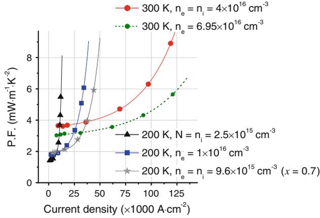
Fig. 5. Power factor as a function of current density for the carrier densities and alloy compositions described in Fig. 2.
