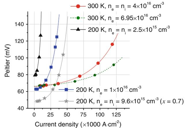
Fig. 4. Peltier coefficient as a function of current density for the carrier densities and alloy compositions described in Fig. 2. Note that the Peltier coefficient of the doped  $\text{InAs}_{0.1}\text{Sb}_{0.9}$  at 300 K in the linear regime is close to that of the intrinsic material.
