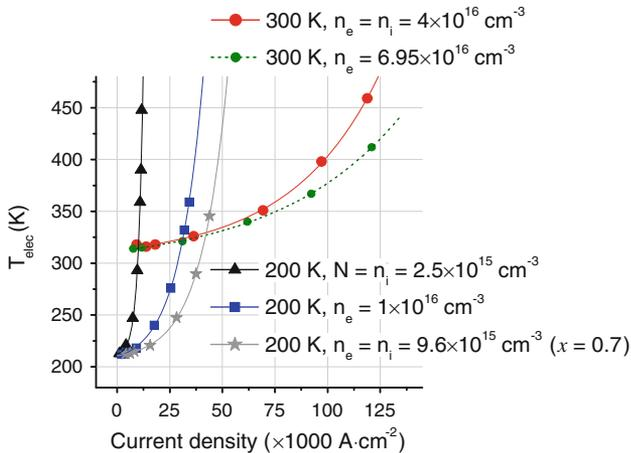
Fig. 3. Electron temperature as a function of current density for the carrier densities and alloy compositions described in Fig. 2.
