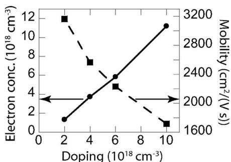
FIG. 4. Room-temperature, in-plane electrical properties of the ErAs:In<sub>0.53</sub>Ga<sub>0.47</sub>As wells as a function of ErAs doping plus silicon codoping. Electron concentration, solid line and filled circles; and electron mobility, dashed line and filled squares.
