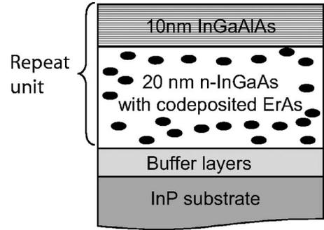
FIG. 3. Schematic diagram of the sample structure. Each sample structure was grown on both semi-insulating substrates for in-plane measurements (30 repeat units) and on conductive ( $n$ -type) substrates (70 repeat units) for cross-plane measurements. Samples were doped with both ErAs and varying amounts of silicon.
