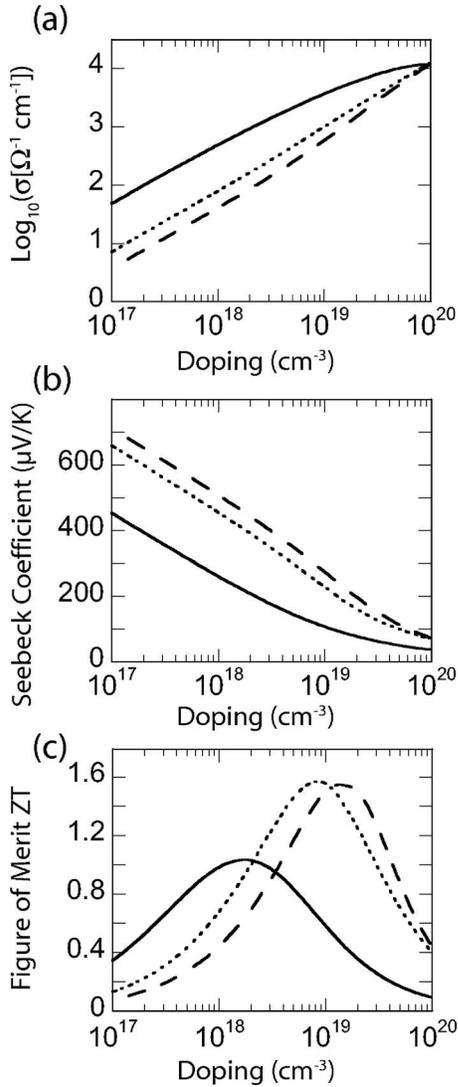
FIG. 2. High-temperature (900 K) modeling of cross-plane electrical and thermoelectric properties: (a) electrical conductivity, (b) Seebeck coefficient, and (c)  $ZT$ . Solid curves are bulk  $\text{In}_{0.53}\text{Ga}_{0.47}\text{As}$ , while dashed curves are superlattices with conserved transverse momentum and dotted curves are superlattices with non-conserved transverse momentum.
