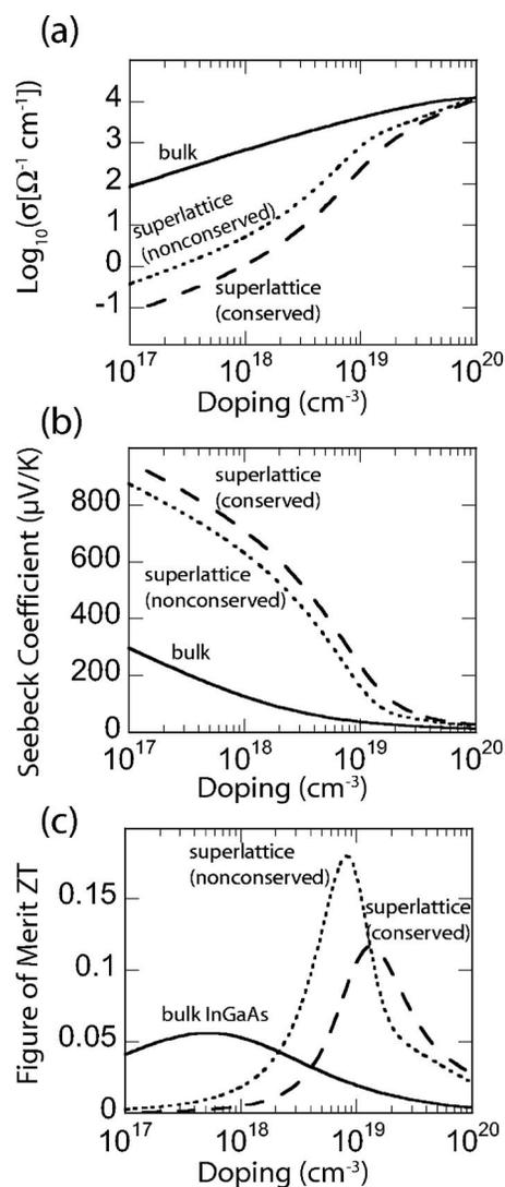
FIG. 1. Room-temperature modeling of cross-plane electrical and thermoelectric properties: (a) electrical conductivity, (b) Seebeck coefficient, and (c)  $ZT$ . Solid curves are bulk  $\text{In}_{0.53}\text{Ga}_{0.47}\text{As}$ , while dashed curves are superlattices with conserved transverse momentum and dotted curves are superlattices with nonconserved transverse momentum.
