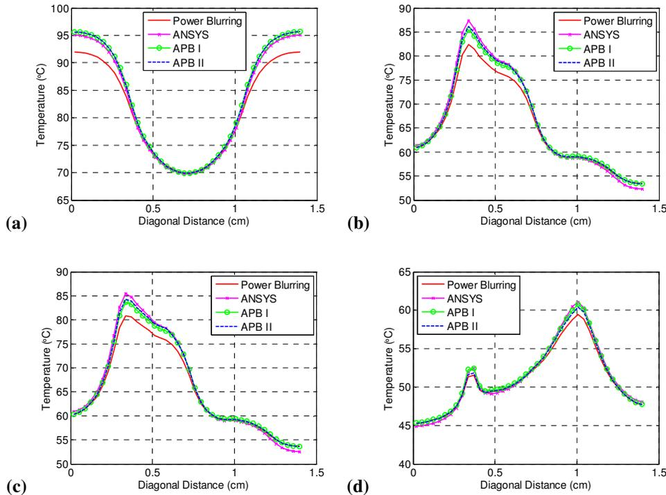
**Figure 7.** Diagonal cross section of the temperature profiles for different power distributions and algorithms. (a) "edge" power map, (b) "μprocessor 1" power map, (c) "μprocessor 2" power map, (d) "μprocessor 3" power map.
