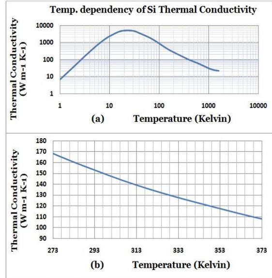
**Figure 1.** Silicon thermal conductivity vs. temperature for a. 0-1500 K, b. 273-373 K (0-100°C).
