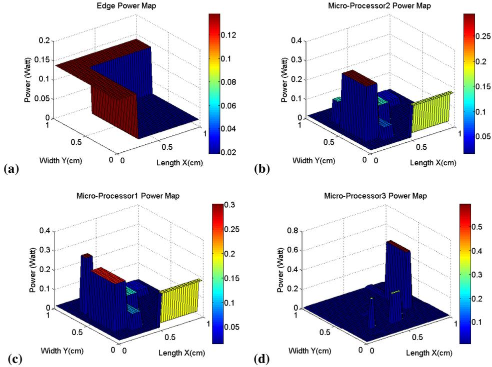
**Figure 5.** 2D view of the four power dissipation maps selected for our study. (a) “Edge” Power map (b) “μprocessor 1” power map (c) “μprocessor 2” power map, and (d) “μprocessor 3” power map.
