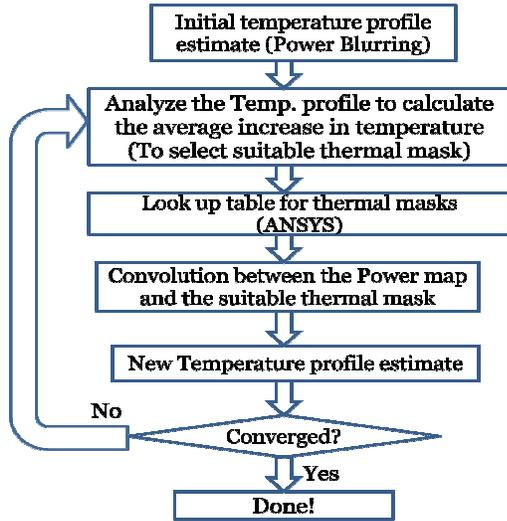
Figure 2. Algorithm for the first Adaptive Power Blurring method (APB\_I).
