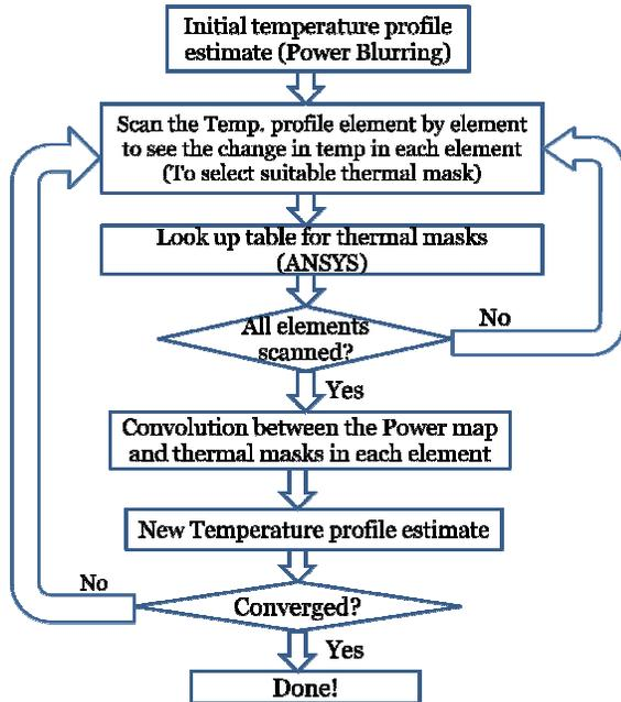
Figure 3. Algorithm for the second Adaptive Power Blurring method (APB\_II).
