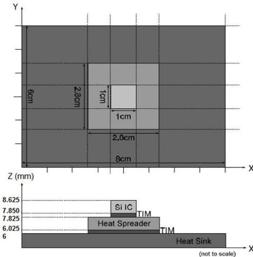
**Figure 4.** Schematic of packaged IC chip and its dimensions
