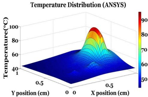
**Figure 6.** Temperature profile obtained from ANSYS for the power map shown in Fig. 5(d).
