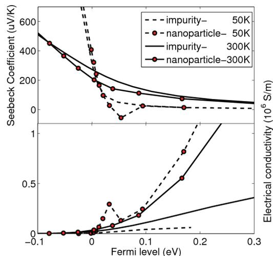
FIGURE 6. Seebeck coefficient (top) and electrical conductivity (bottom) versus Fermi level for impurity and nanoparticle doped samples at 50 and 300 K. Samples are described in the text.
