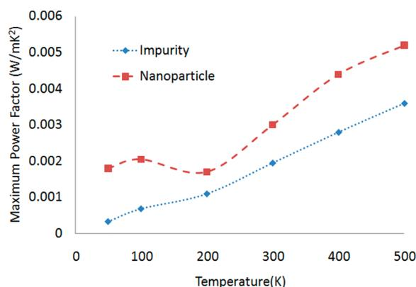
**FIGURE 5.** Maximum thermoelectric power factor versus temperature for the nanoparticle-doped GaAs compared to the impurity-doped GaAs. At each temperature, the power factor was maximized versus Fermi-level. Modeling is performed for GaAs with 5% volume fraction of 0.2 eV height nanoparticles. Band bending of the nanoparticles are included. Phonon scattering rates (polar optical and acoustic) are also included in the calculations. Refer to text for other properties.
