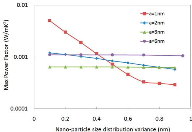
**FIGURE 3.** Maximum power factor versus nanoparticle size variance. Different curves refer to different average radius ( $a$ ) of nanoparticles. In this curve, we assumed a 5% nanoparticle volume fraction and 0.5 eV nanoparticle barrier height.
