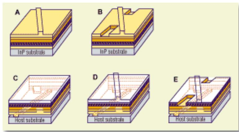
Figure 4 Fabrication steps for an x-crossing coupler include (a) forming the upper waveguide, (b) removing the InGaAsP layer, (c) inverting the sample to bond to a host layer and to remove original substrate and etch stop layer, (d) fabricating another waveguide, and (e) removing the InGaAsP layer.
