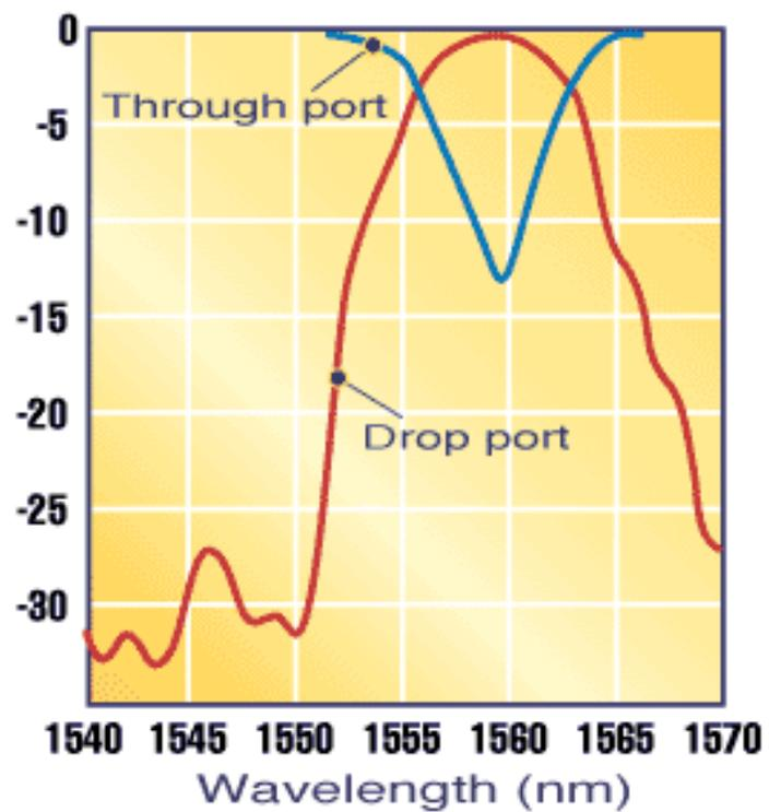
Figure 5 Transmission spectra of the TE mode shows a 3-dB bandwidth of 6 nm. Data have been normalized to the total
