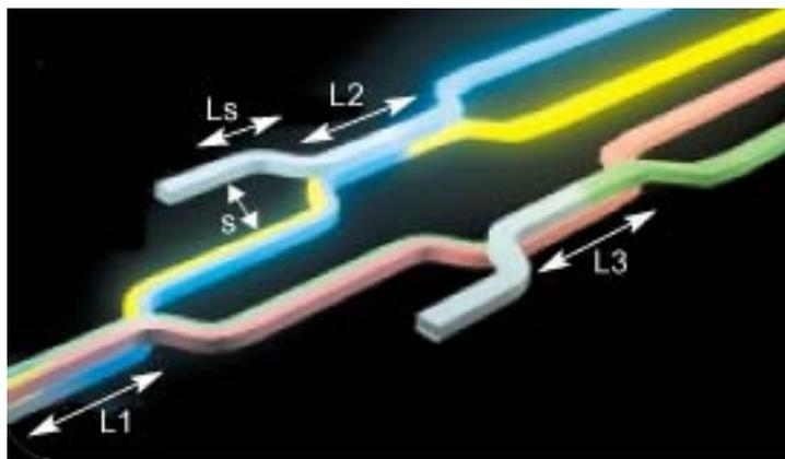
*Figure 1 A four-channel multiplexer incorporates a pair of 3-D vertical couplers. Vertical coupler  $L_1$  is 5 mm,  $L_2$  is 2.397 mm, and  $L_3$  is 2.37 mm. The horizontal spacing  $S$  is 10  $\mu\text{m}$ , and the length of the S-bend  $L_s$  is 500  $\mu\text{m}$ .*
