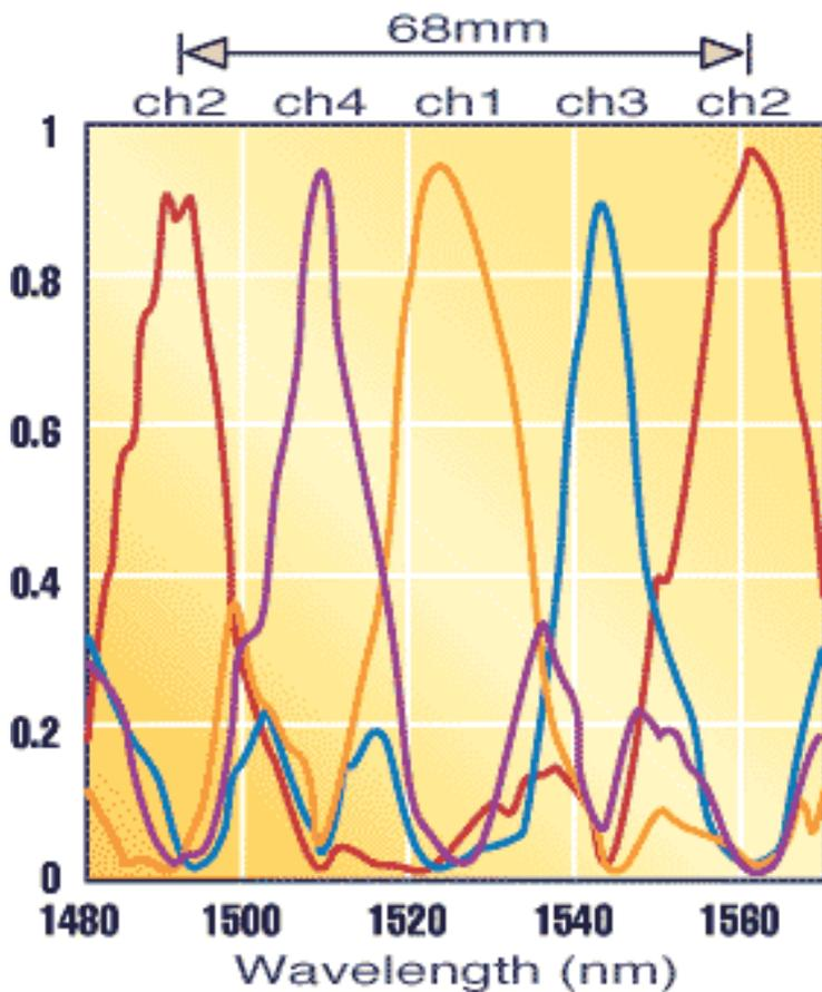
*Figure 3 Output light intensity as a function of wavelength for the four channels shows a free spectral range of 68 nm.*
