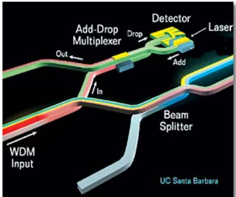
*Figure 6 Wafer fusion techniques can integrate active and passive devices.*
