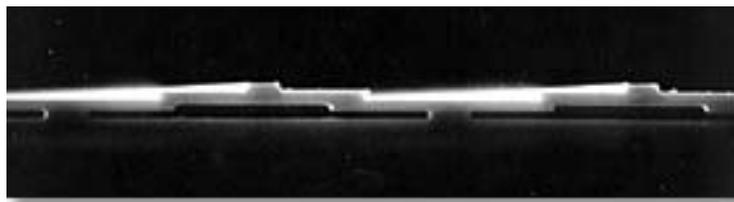
*Figure 2 A scanning-electron-microscope (SEM) image shows the output facet of a four-channel MUX/DEMUX.*
