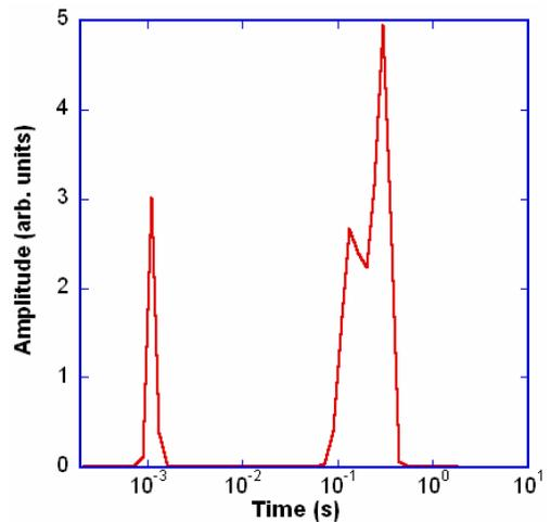
**Figure 3:** Time constant spectrum of the whole studied device.
