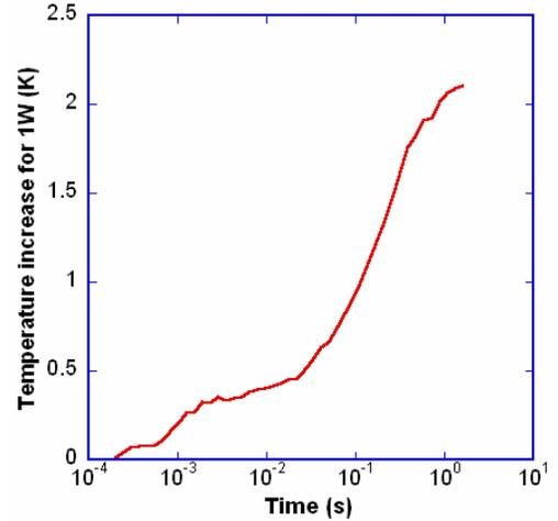
**Figure 2:** Measured temperature transient response of the whole device when the later is supplied by a step excitation current of 1W.
