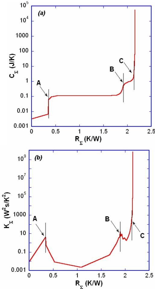
**Figure 4:** (a) Cumulative structure function and (b) differential structure function of the whole studied device.
