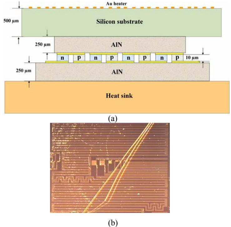
**Figure 1:** Schematic diagram of the ErAs: InGaAs/InAlAs thermoelectric power generator.
