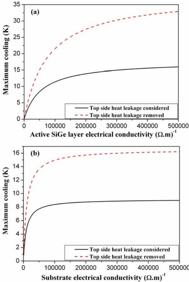
**Figure 7:** Calculated maximum cooling of a  $50 \times 50 \mu\text{m}^2$  device with  $10 \mu\text{m}$  thick SiGe layer as a function of the active SiGe layer electrical conductivity (a) and the substrate electrical conductivity (b). In each case, the solid line corresponds to the current realistic device with top side heat leakage, and the dashed line corresponds to the case without top side heat leakage.
