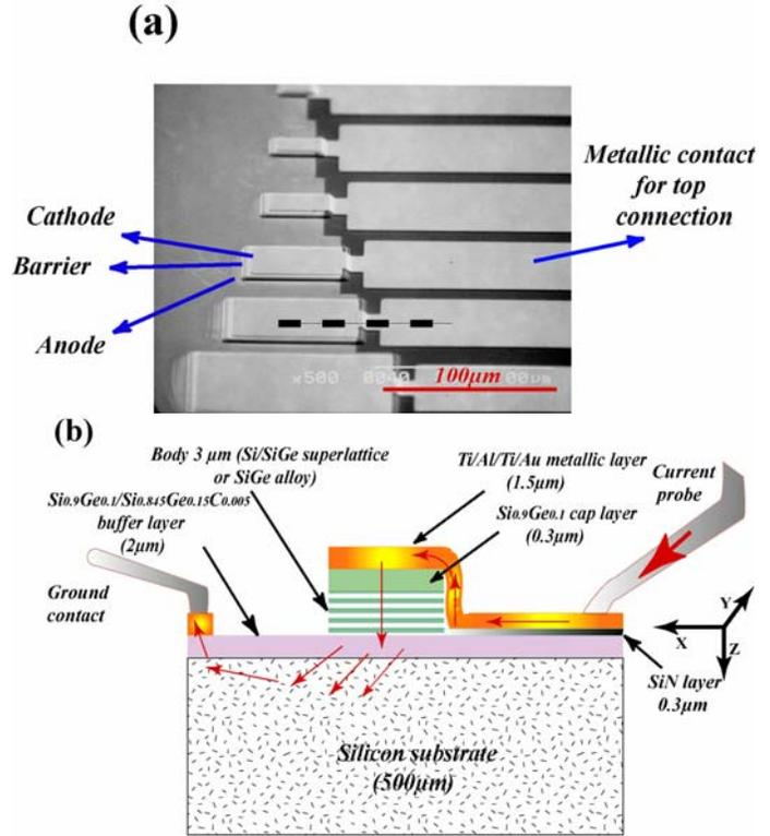
**Figure 1:** (a) SEM picture of a set of microrefrigerators with five different sizes, and (b) Schematic diagram of the microrefrigerator cross sectional view. Arrows indicate the direction of the electron flux. X is the direction of the metal lead at the top side, Z is the cross plan direction, and Y is the complementary direction.
