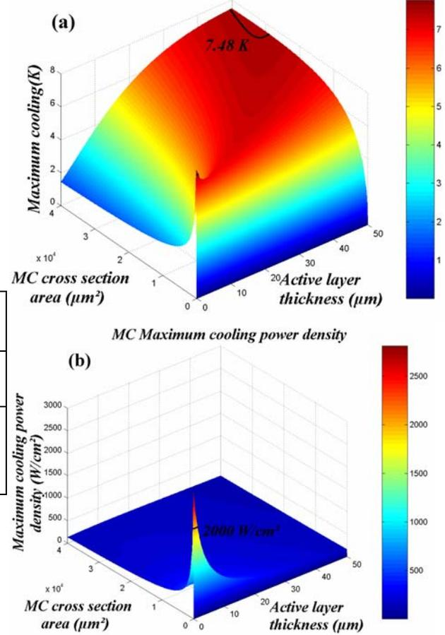
**Figure 4:** Calculated microrefrigerator maximum cooling (a) and maximum cooling power density (b) as a function of the microrefrigerator cross sectional area and the active SiGe layer thickness. In figure (a), the black contours show the maximum cooling value within the range of the used variables, and in figure (b), the black contour show a particular value of  $2000 \text{ W/cm}^2$  just as a reference.
