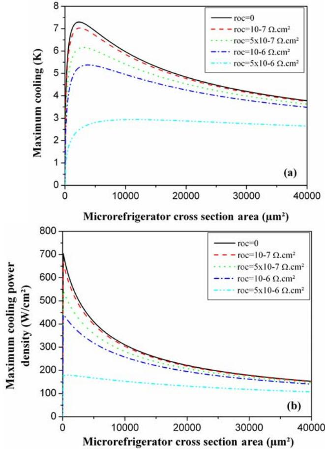
**Figure 5:** Calculated maximum cooling (a) and the maximum cooling power density (b) as a function of the device cross section area for different Ohmic contact resistances values.
