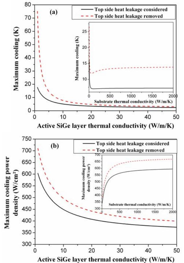
**Figure 6:** Calculated maximum cooling (a) and maximum cooling power density (b) of a  $50 \times 50 \mu\text{m}^2$  device with  $10 \mu\text{m}$  thick active SiGe layer as a function of the active SiGe layer thermal conductivity and the substrate thermal conductivity (the inset). In each case, the solid line corresponds to the current
