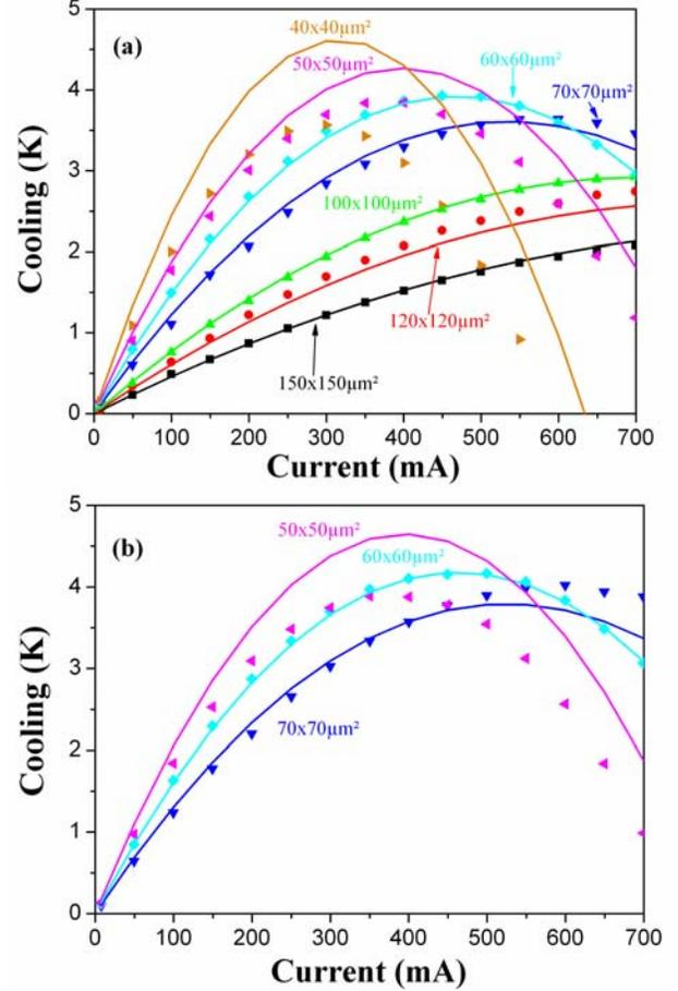
**Figure 3:** Measured cooling on thin film bulk SiGe microrefrigerator (a) and Si/SiGe superlattice microrefrigerator (b) for different device sizes, and their corresponding fit based on Thermal Quadrupoles Method.
