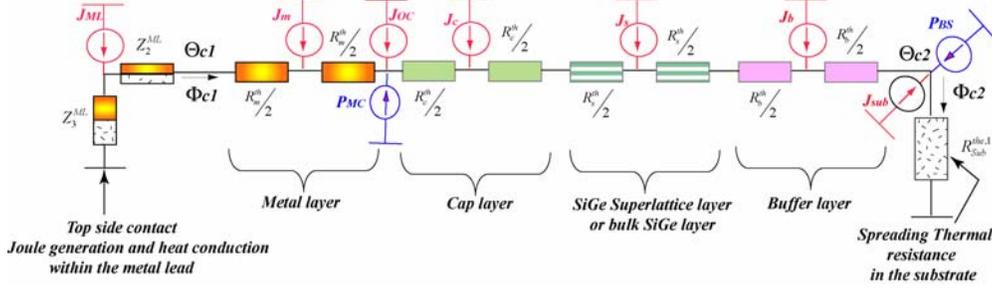
**Figure 2:** Thermal quadrupole network associated with the heat transfer within the whole SiGe microrefrigerator in a steady state regime
