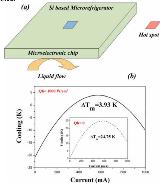
**Figure 10:** (a) Schema of the model configuration for combining microrefrigerator cooling with liquid cooling. (b) Variation of the microrefrigerator cooling as a function of the applied current for a heat load of  $1000\text{ W/cm}^2$ , in comparison with the case of zero heat load (the inset).
