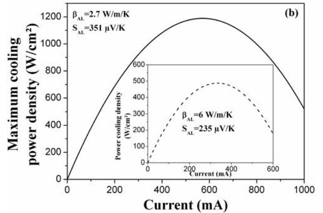
**Figure 9:** Calculated microrefrigerator cooling (a) and maximum cooling power density (b) as a function of the applied current when the active layer figure of merit  $ZT$  is increased by a factor of 5. The insets show the performance curves for the current devices.
