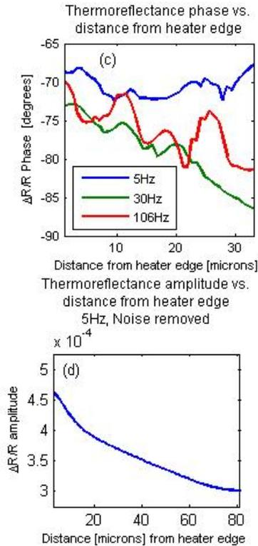
**Figure 5:** (a) Thermoreflectance image of the heater line on top of the InGaAs thin film sample.  $\Delta R/R$  amplitude (b) and phase (c) profiles perpendicular to heater for frequencies 5, 30, and 106 Hz. Smoothed  $\Delta R/R$  amplitude profile at 5 Hz.
