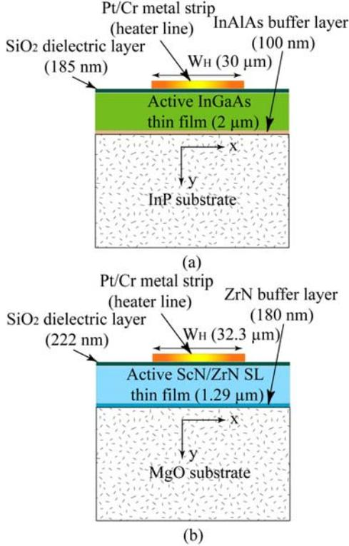
**Figure 1:** Schematic diagram of the two test structures studied; the isotropic InGaAs thin film on the isotropic InP substrate (a), and the anisotropic ScN/ZrN superlattice thin film on the isotropic MgO substrate (b).
