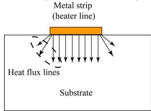
**Figure 3:** A sketch illustrating the effect of width of the metal heater strip on the heat flux path in a  $3\omega$  system.
