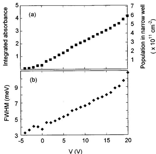
FIG. 3. Absorption characteristics of the narrow well as a function of external bias at  $T = 10$  K. (a) The integrated absorbance and population in the narrow well vs external bias. (b) FWHM vs external bias.
