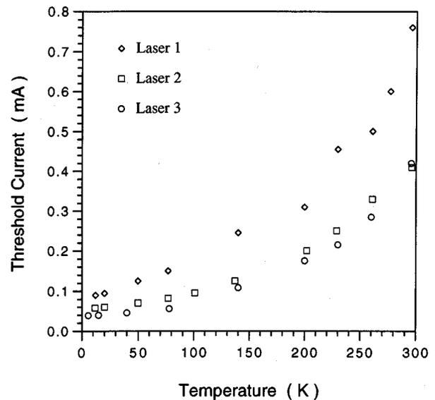
FIG. 1. Measured threshold current as a function of ambient temperature for 225- $\mu\text{m}$ -long InGaAs strained single quantum well buried heterostructure lasers. The lasers have different mirror facet coatings. See Table 1 for the detail.
