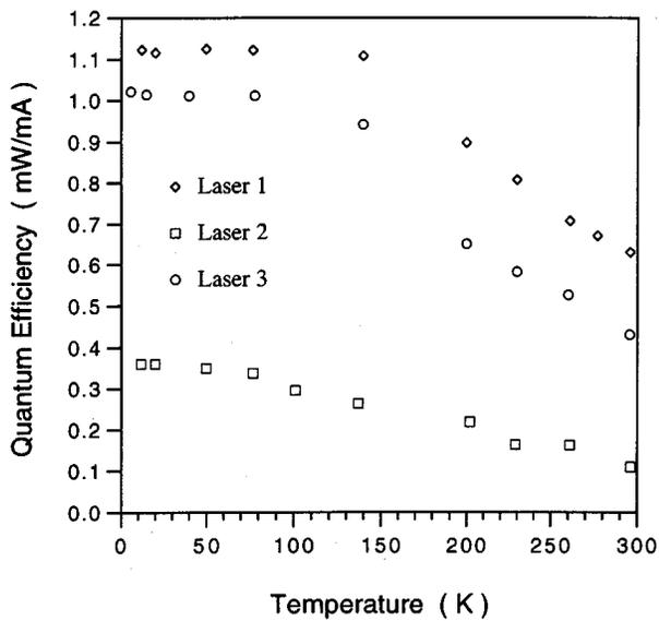
FIG. 2. Measured external quantum efficiency as a function of ambient temperature for 225- $\mu\text{m}$ -long InGaAs strained single quantum well buried heterostructure lasers. The lasers have different mirror facet coatings. See Table I for the detail.
