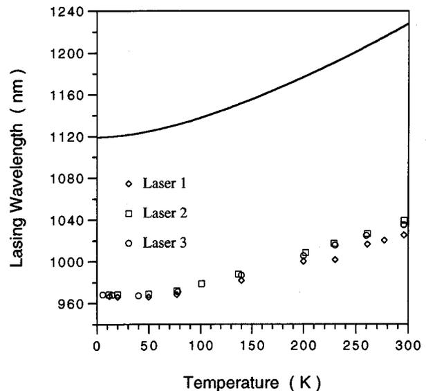
FIG. 4. Measured lasing wavelength as a function of temperature in the strained InGaAs SQW lasers. The solid line is the calculated wavelength corresponding to the  $\text{In}_{0.3}\text{Ga}_{0.7}\text{As}$  energy band gap.
