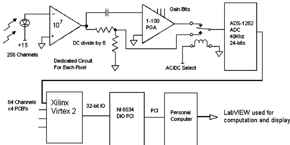
FIG. 1. Single pixel flow of the UCSC thermoreflectance thermal imaging system.
