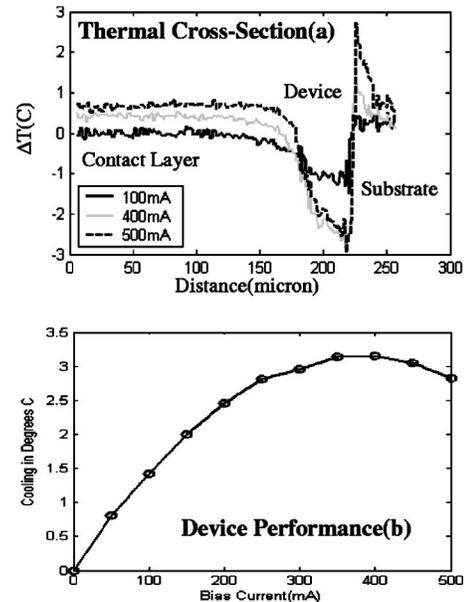
FIG. 9. Quantitative analysis: Average surface temperature (a) and cross sections (b) of active  $50 \times 50\ \mu\text{m}$  microcooler. Ten images of the microcooler at increasing bias current show a maximum surface cooling of 3.2 from 30 C stage temperature. Cross sections down the contact layer to the microcooling surface shows good cooling distribution on the device but too much heating on the substrate around the device.
