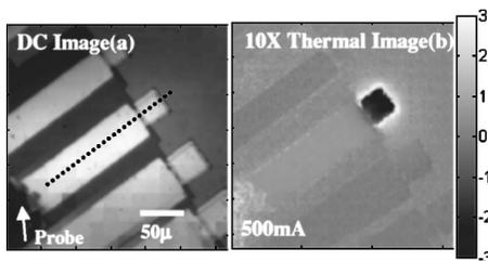
FIG. 8. Typical results: dc image (a) and thermal image (b) acquired on a  $50 \times 50\ \mu\text{m}$  SiGe microcooler biased at 500 mA, 30 C stage temperature. This device is limited by heating on the substrate, probably due to too much resistance between the superlattice and buffer layer. The dotted line is the cross section used in the following figure.
