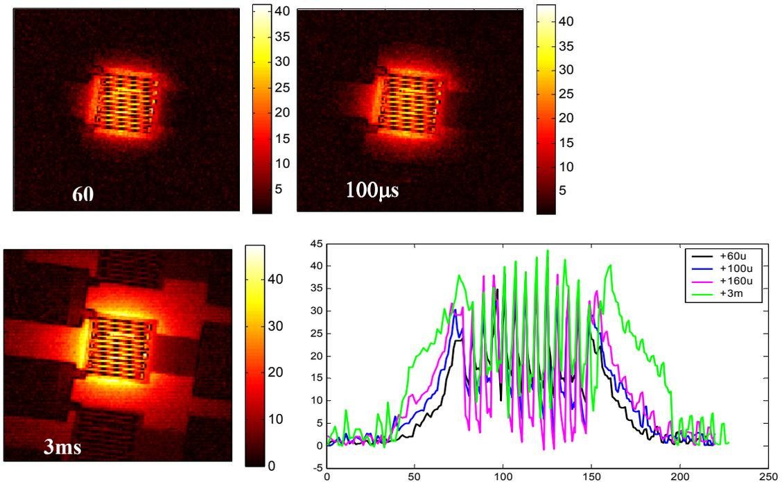
**Figure 4:** Long time scale (ms) response of 100 micron heater showing slower heat diffusion in the substrate. Thermal images are in  $\Delta T$  (degrees C).
