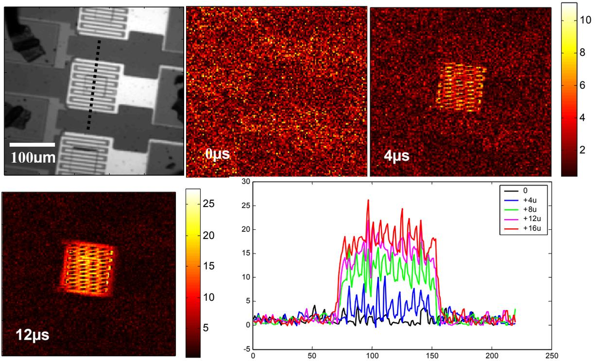
**Figure 3:** Short timescale response of 100 micron heater showing rapid heat diffusion on the device metal. Thermal cross sections are indicated by the dotted line. Thermal images are in  $\Delta T$  (degrees C).
