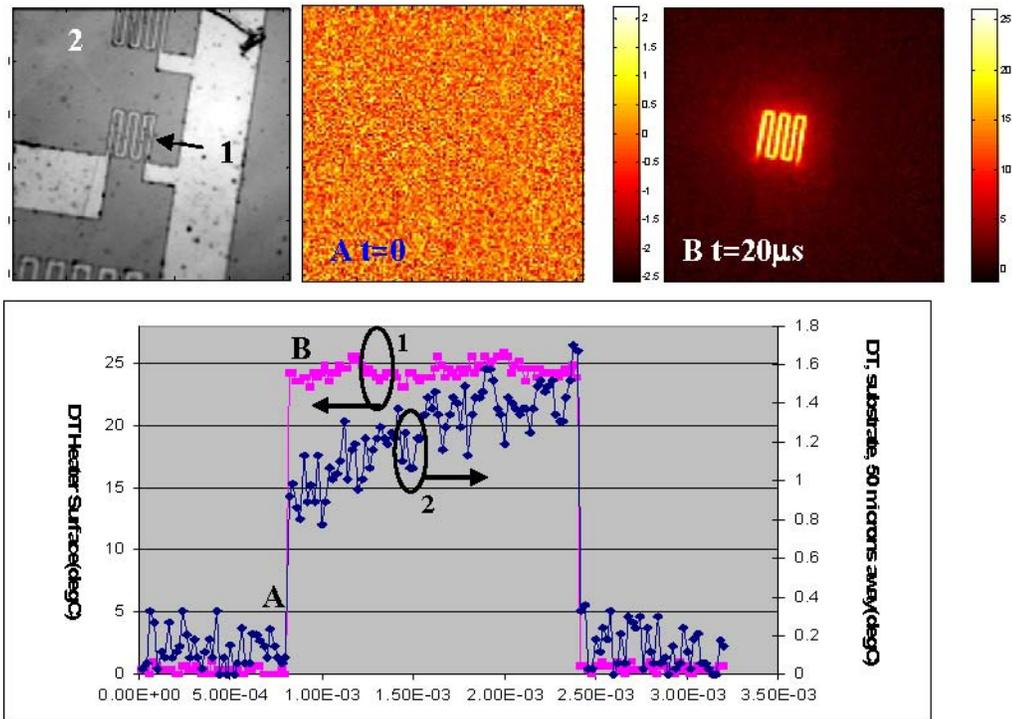
**Figure 2:** Time series of data point on heater (1), and data point 50 microns away (2) on the substrate. The device metal has faster heat diffusion and achieves uniform heating more rapidly
