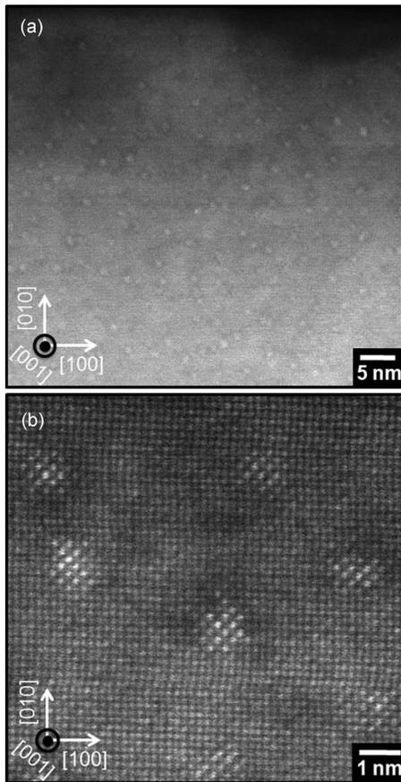
FIG. 4. (a) HAADF STEM plan-view images of self-assembled TbAs nanoparticles in GaAs grown on (001) GaAs and viewed along the  $[00\bar{1}]$  direction. The TbAs concentration of the layer was approximately 1.8%, and the average particle diameter was approximately 1.5 nm. (b) The rocksalt crystal structure of TbAs and continuous As sublattice throughout the sample are visible. TbAs appears bright in the images.
