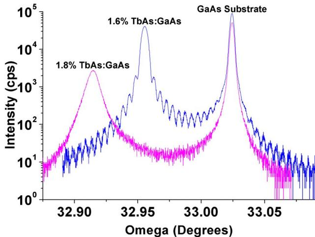
FIG. 1. (Color online)  $\omega$ - $2\theta$  XRD rocking curves of two TbAs:GaAs samples found to have 1.6% and 1.8% TbAs concentrations. Fringes on the 1.6% sample were used to calculate film thickness, and the FWHMs of the film peaks indicated good crystallinity.
